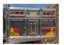
• Tailgate hinge configuration, operable from the ground
