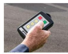
Remote control for tipper operation (High Volume Side Tipper)
