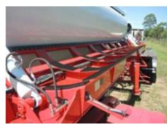
• 5 ply rubber wear pads to chassis
