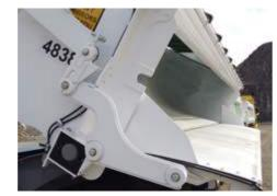
Mechanical arm with over centre lock (Door Side Tipper)
